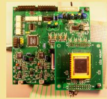
Figure 6. CCD & TDI control board
