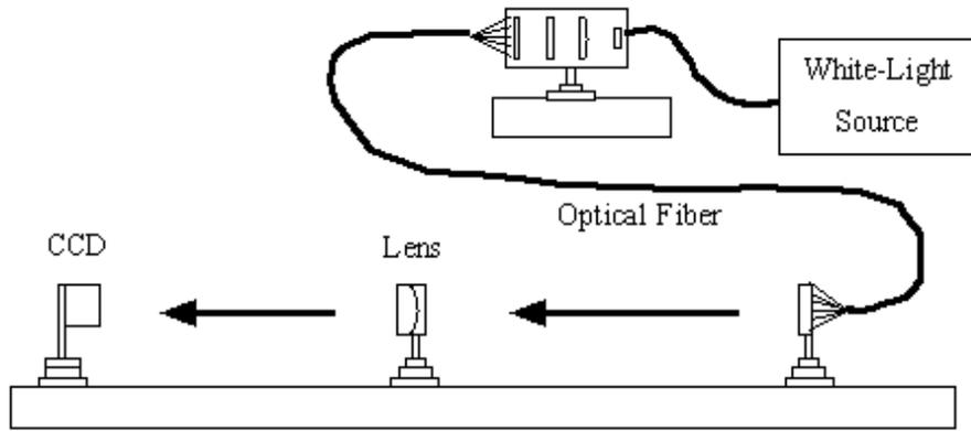
Figure 5. Centroiding Experiment Layout
