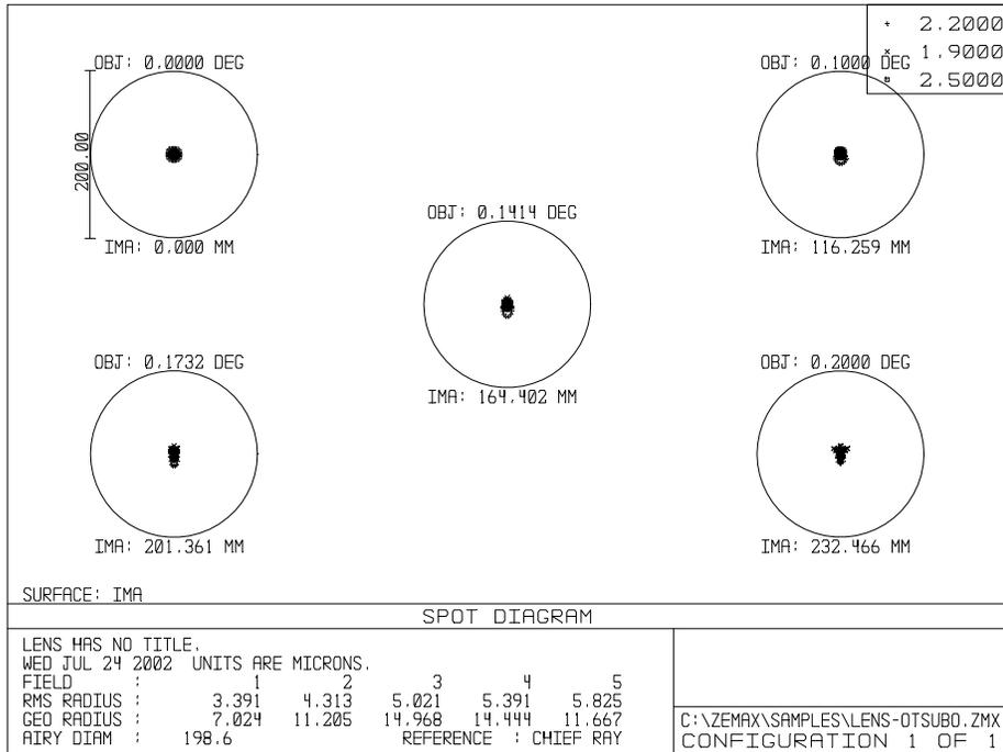
Figure 4. Spot Diagram in the optical configuration for JASMINE-I.
