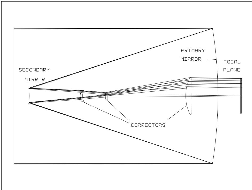
**Figure 3.** Optical configuration of the astrometric instrument for JASMINE-I. The optical system is optimized for the astrometric measurement in K-band.
