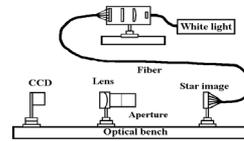
Fig. 1 Schematic of the Experimental Equipment
